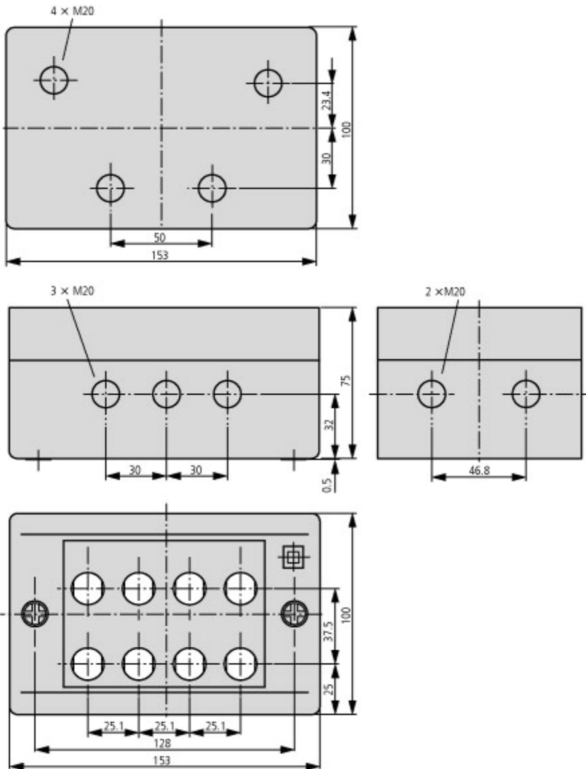
Fixing holes: 2 x  $\varnothing$  4.5 mm
