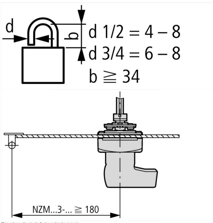
Minimum door coupling rotary handle clearance from door pivot point
