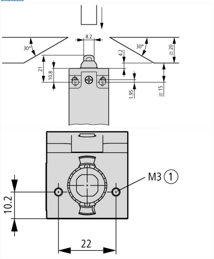
① screw-in depth max. 12 mm
