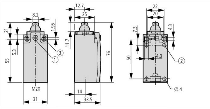
$\begin{array}{l} (1) \mbox{ Tightening torque of cover screws: 0.8 Nm \pm 0.2 Nm } \\ (2) \mbox{ only with LS (insulated version)} \\ (3) \mbox{ Fixing screws 2 x M4 } \geq 30 \\ M_{\rm A} = 1.5 \mbox{ Nm} \end{array}$
